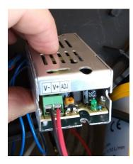
Fix the power supply to the bottom support bracket using the bihadesive tape
